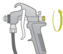
Open Restrict Paint Control knob by turning counter clockwise.
